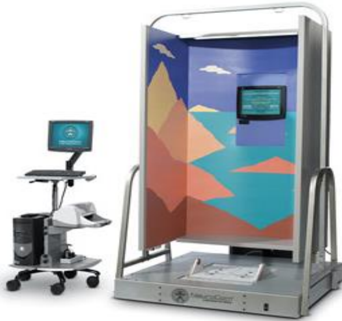
Figure 1A. Computerized Dynamic Posturography Sensory Organization Test (SOT)
